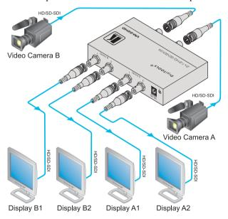
Figure 2: Connecting the VM-22HD in Single Link Mode
