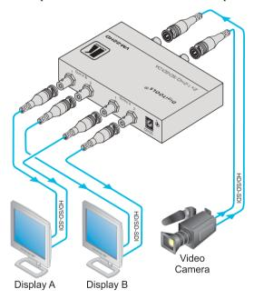
Figure 3: Connecting the VM-22HD in Dual Link Mode
