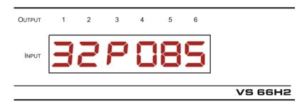
In this example: Input 3 is routed to output 1, input 2 is routed to output 2, a pattern is routed to output 3, output 4 is set to mute, and so on.
